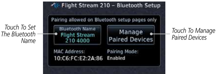
Bluetooth Setup for Flight Stream 210
